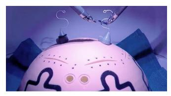
surgery). This task trains camera navigation, effective use of the camera clutch, and wristed instrument maneuvering for precise instrument tip positioning.
